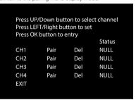
■ Use buttons C⑦ and C⑨ to select your preferred channel (CH1 to CH4). Use buttons C⑭ and C⑪ to select item "Pair" (pair). Confirm the selection by pressing the button Menu/OK C⑨. The message "Pairing..." (pairing) will appear on the screen C⑨. If the pairing process is successful, the message "Pairing succeed, CHx is selected. Press OK button to back Menu." will appear on the screen C⑨. After a moment, the screen C⑨ will automatically switch to the picture from camera B⑨ display mode.
