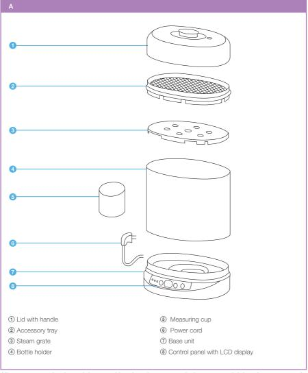
All parts, except for the stainless steel heating plate, are made from a material that does not contain BPA (Bisphenol A).
